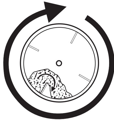
Figure 2. Fin structure in barrel composter.
