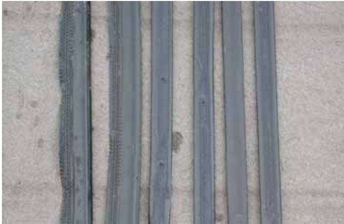
Figure 3. Drip tapes can be distinguished and recognized by their features. Note the emitter (on the four tapes on the right) and the turbulent flow channels (on the two tapes on the left). Credits: Eric Simonne.
