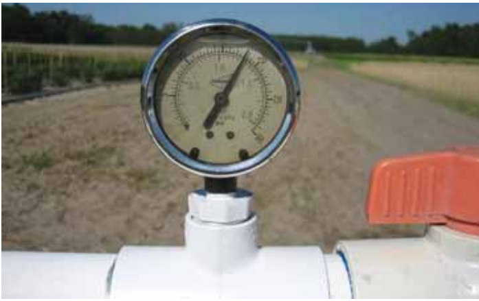
Figure 10. A fixed pressure gauge. Note the needle bathing in oil to prevent needle vibration and damage. Credits: Eric Simonne.
