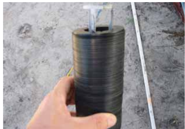
Figure 6. Disk filters are made of stacked disks with small openings. They are usually color coded to indicate the filtration mesh. Credits: Eric Simonne.
