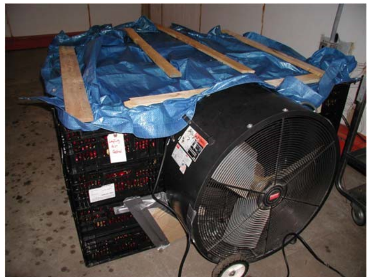
Figure 68: Air is drawn through the wrapped pallet with a fan to create a homemade, but effective, forced air cooling system helping to improve shelf life.
